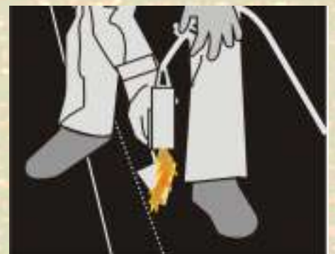
Using A Trowel To Seal Overlaps.
